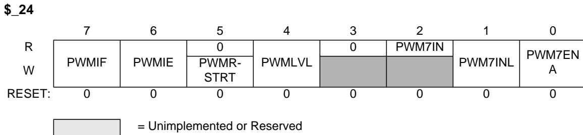
Figure 3-15 PWM Shutdown Register (PWMSDN)
