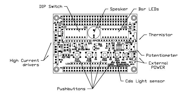
The demo program will monitor the state of the DIP switch position, the analog values of potentiometer, thermistor, and Cds light sensor as percentage of full scale. As well, the high current drivers and Bar LEDs can be controlled to be turned off or on via PC keyboard.
