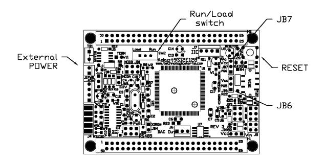
Make sure to connect Adapt9S12E128 H2 to LAN card P2 header. H1 and P1 maynot have to be connected. It is all dependent whether the boards are stacked or in a planar arrangement.
