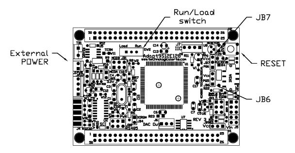
To start, slide Run/Load switch to Load, power up the board then press the RESET pushbutton momentarily. Double click on the uBUG12 icon to execute uBUG12 program. In the command bar type "con 1" (without the double quote) for COM 1 and "con 2" for COM 2. A "connect" message will appear in the uBUG12 window to indicate that PC and Adapt9S12E128 established communications.
