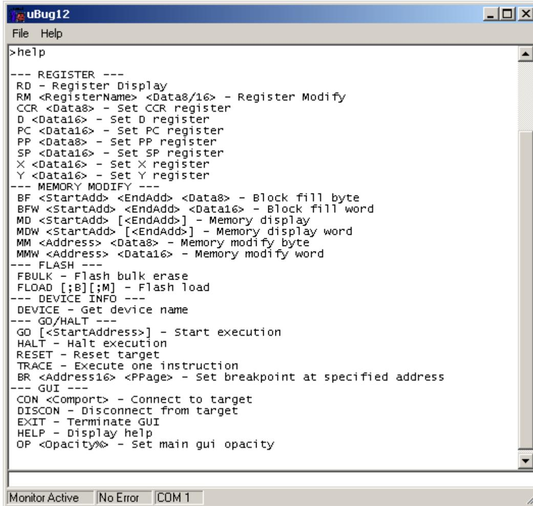
The screenshot shows a window titled "uBug12" with a menu bar containing "File" and "Help". The main area displays the output of the "help" command, which lists various debugging commands and their syntax. The commands are grouped into categories: REGISTER, MEMORY MODIFY, FLASH, DEVICE INFO, GO/HALT, and GUI. At the bottom of the window, there are three status indicators: "Monitor Active", "No Error", and "COM 1".
