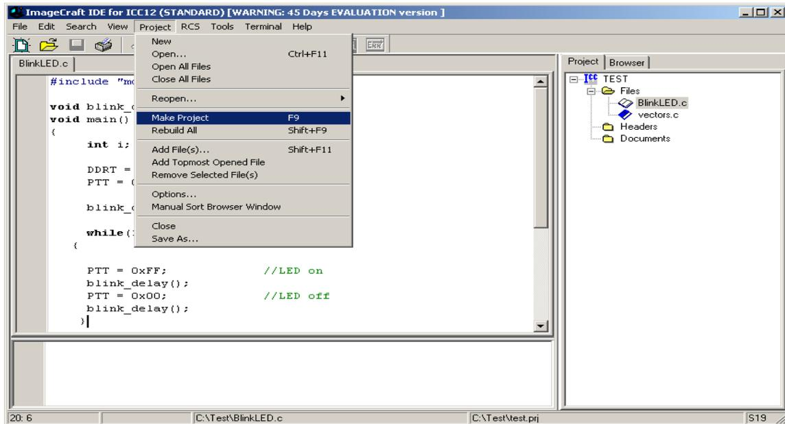
Note the bottom window pane will show messages to display how the build progressed. Any errors, if any, are shown in this window. The build was without error so we can progress to erasing and programming the 9S12C32.
