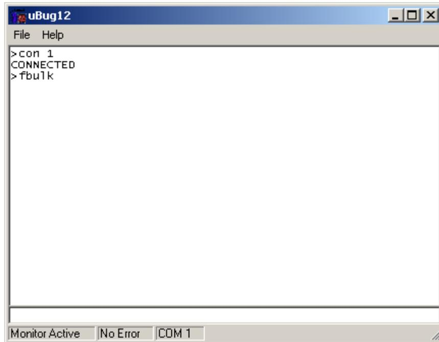
To program, type the command **FLOAD ;B** for banked S19, S2, SX and formatted S19 (went thru SrecCVT program) records. For non-banked S2 the command is **FLOAD**.
