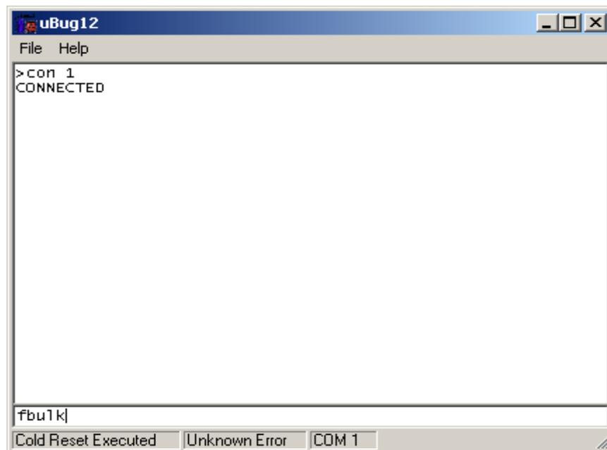
Make sure to erase the FLASH memory by typing the command **FBULK**.
