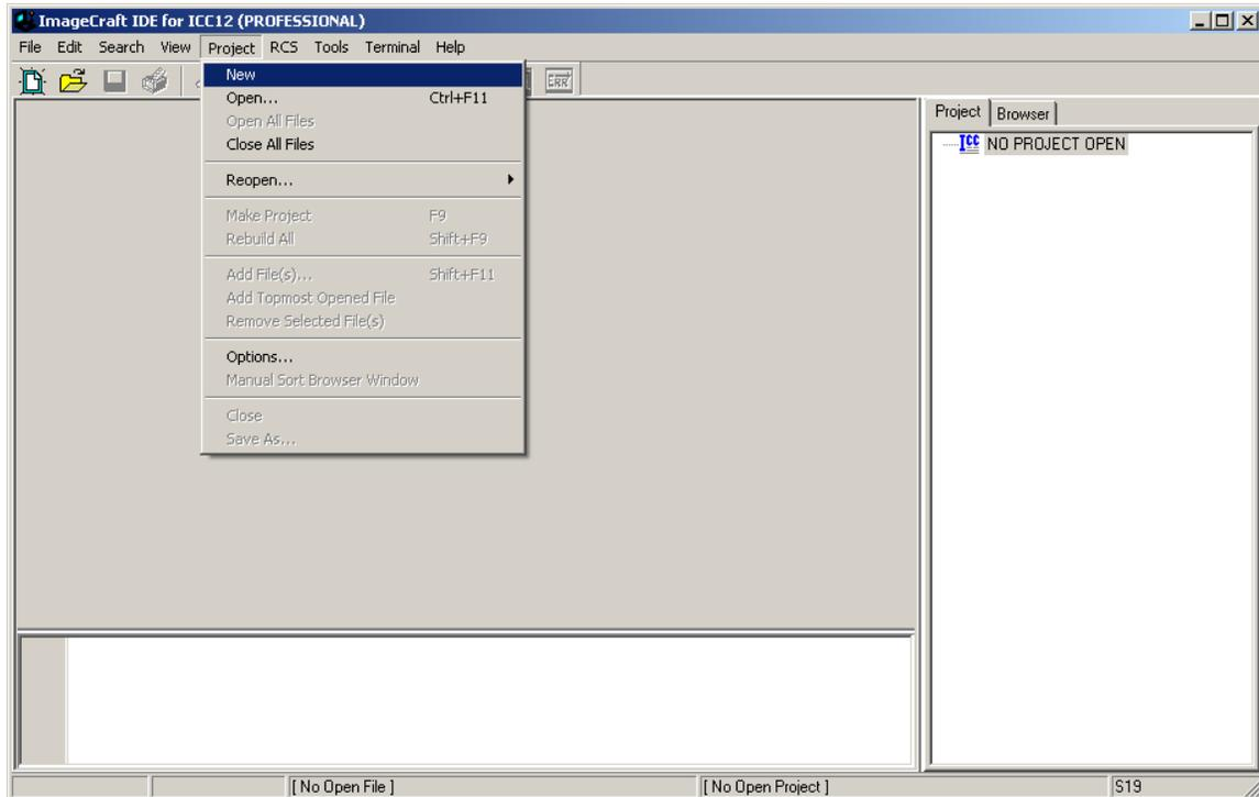
The ICC12 will prompt to save the new project. The user should decide whether to create a new directory to save the new project. In this example a new directory called **Test** is created and the file is saved as file **test.prj**.
