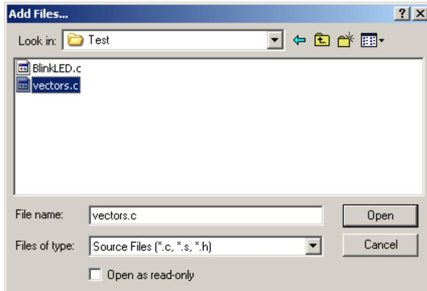
Note that ICC12 has changed to include **vectors.c**. It is important to note that the **vectors.c** was written for the 68HC912B32 and 812A4 MCUs. One should edit the file to include other ISR addresses for the 9S12C32. This example uses the file as is.
