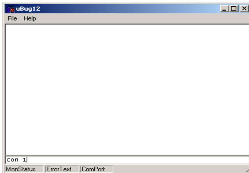
In the command bar type **con 1** for COM 1 or **con 2** for COM 2. A **CONNECTED** message will appear to indicate that a connection between PC and NC12 has been established.
