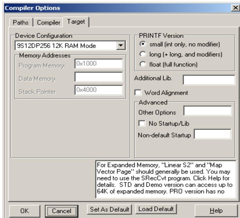
Scroll up or down to select Custom as shown. Note that an 9S12C32 device Configuration does already exist. Unfortunately, the addresses are not setup properly with using uBUG12. Therefore the Custom configuration must be selected and the memory parameters are changed to reflect uBUG12 usage.
