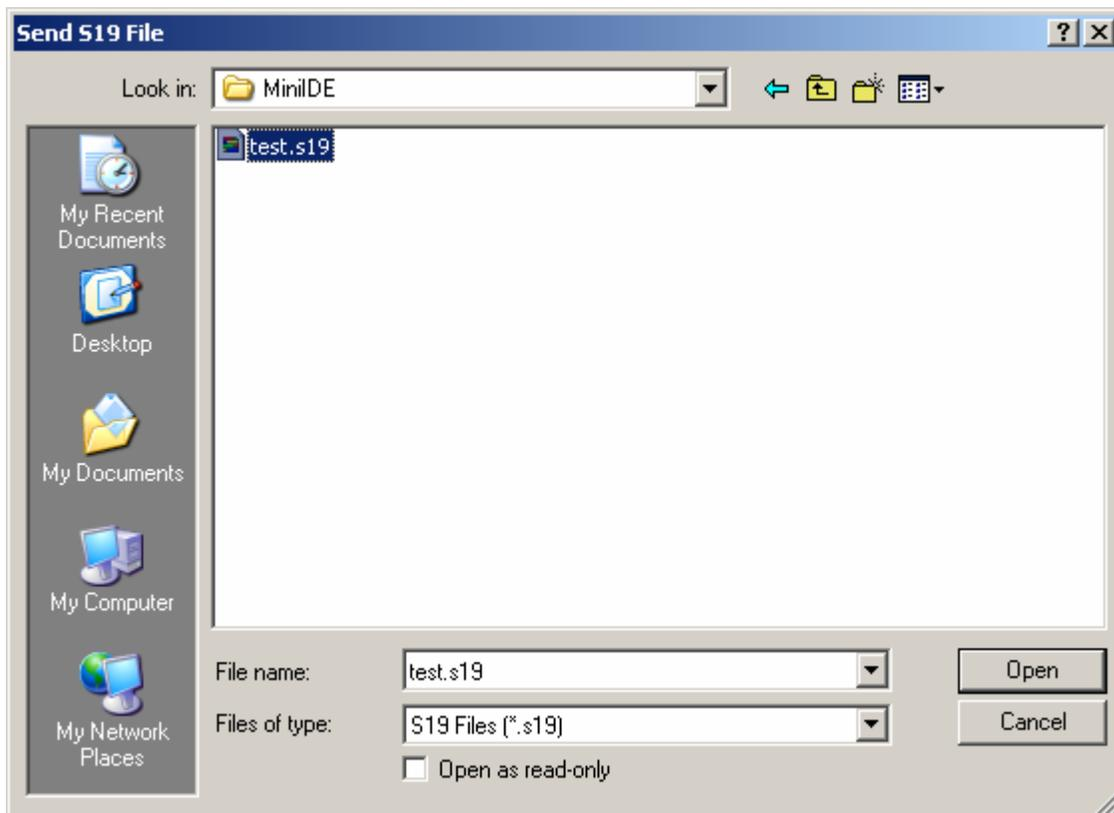
A warning message will pop to prompt in making sure the Run/Boot switch is in Boot mode and the write protect switch is in write position. For Adapt11C24DX SW2 should be positioned to boot and SW4 to write position. Press the RESET button once these are configured. It is assumed that the module is powered up with known good power supply. Press the OK button to initiate program of EEPROM.
