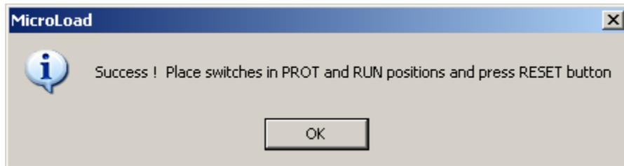
Slide SW4 to protect and SW2 to Run. Press the RESET button and the LED should now blink.
