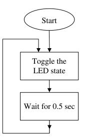
As you saw, the half-second delay caused the LED to blink at a rate of approximately 1 cycle/sec (ignoring the few clock cycles needed to jump back to the top and toggle the LED state). Now let's analyze the code to see how that was accomplished.
