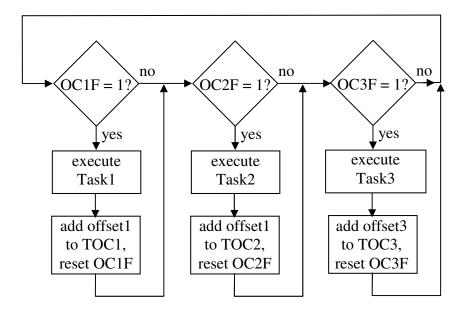
In this experiment you will be using TCNT and three Output Compare registers to execute three tasks at different frequencies. Here is a high-level description of the three tasks:
