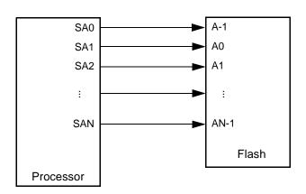
Figure 2. Byte Address Processor Connected to Byte Mode x8/x16 Flash
